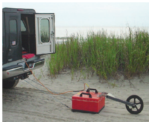
Where access was available, the GPR antenna was towed behind a truck. It has an attached survey wheel, which triggers the recording and measures distance. Photograph by Wayne Baldwin .
