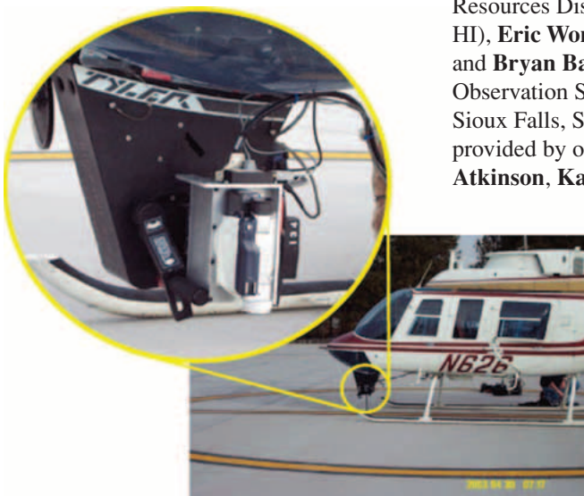
The Duncan Tech MS3100 camera system is mounted beneath a helicopter, using an industry-standard Tyler mount.
