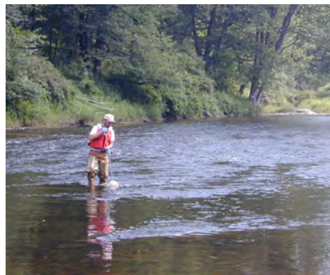
Figure 5. USGS hydrologist collecting a depth-integrated water-quality sample.
