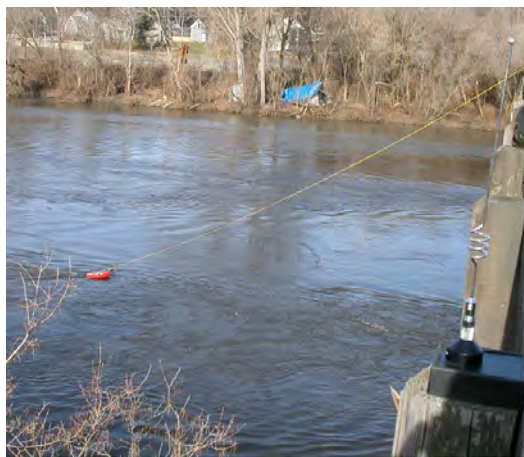
Figure 3. Using an Acoustic Doppler Collection Platform to measure streamflow in a river.
