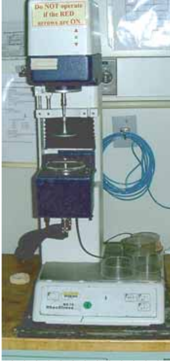
Rheometers provide useful information about the risk of early or late stiffening and setting.
