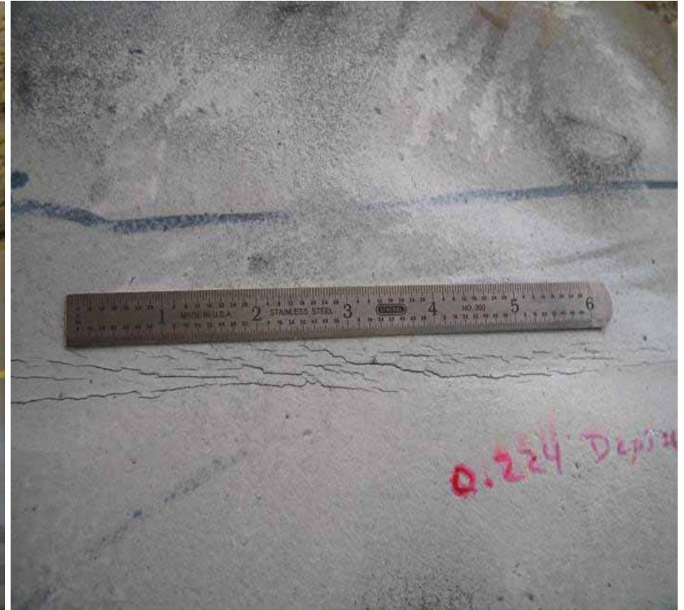
Top of Pipe Mechanical Damage/Gouge Multiple Dents
