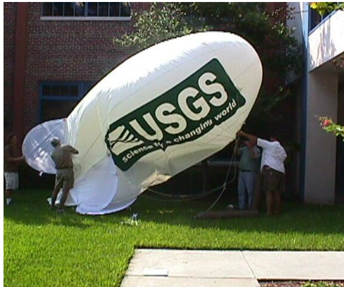
Gene's Shinn's 24-ft-long blimp designed to sample African dust.
