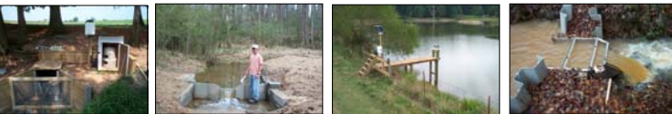
W2 Spring Flume Pond Inflow Weir Pond Level Sensor Pond Outflow Weir
