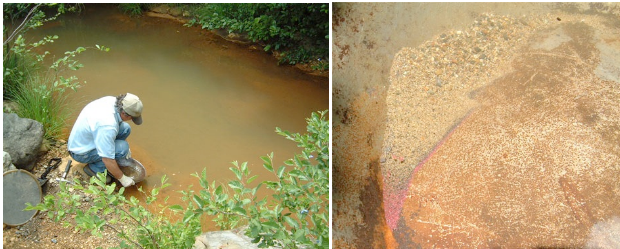
Figure 14. (a) James Creek at sample site 04JC1. Sediment consists of medium to coarse sand and fine silt to clay sizes, the latter containing iron (hydr)oxides derived from Corona and Twin Peaks mine drainage. (b) Cinnabar present in panned concentrate from this location.
