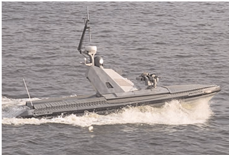
The Protector, manufactured by BAE Systems, Lockheed Martin and Rafael Armament Development Authority, Ltd., is a remote-controlled Unmanned Surface Vehicle (USV) equipped with a stabilized mini-Typhoon weapon system (MK 49 Mod 0), cameras, radar equipment and electro optics.
