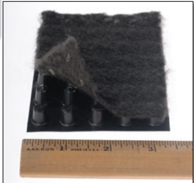
Figure 7—Geocomposites such as sheet drains have a large cross section that allows drainage. If geotextiles are placed under the trail tread, the sheet drain should be oriented with the geotextile on the bottom and the plastic core on top. This orientation reduces the amount of fill needed.
