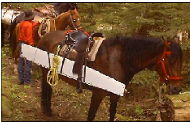
Figure 32—A rigid saw sheath configured for a riding saddle. This design also could be sized for a shorter saw, or used on a pack animal.—Photo used with permission of Jim Thode, Lewis County Chapter of the Backcountry Horsemen of Washington.
