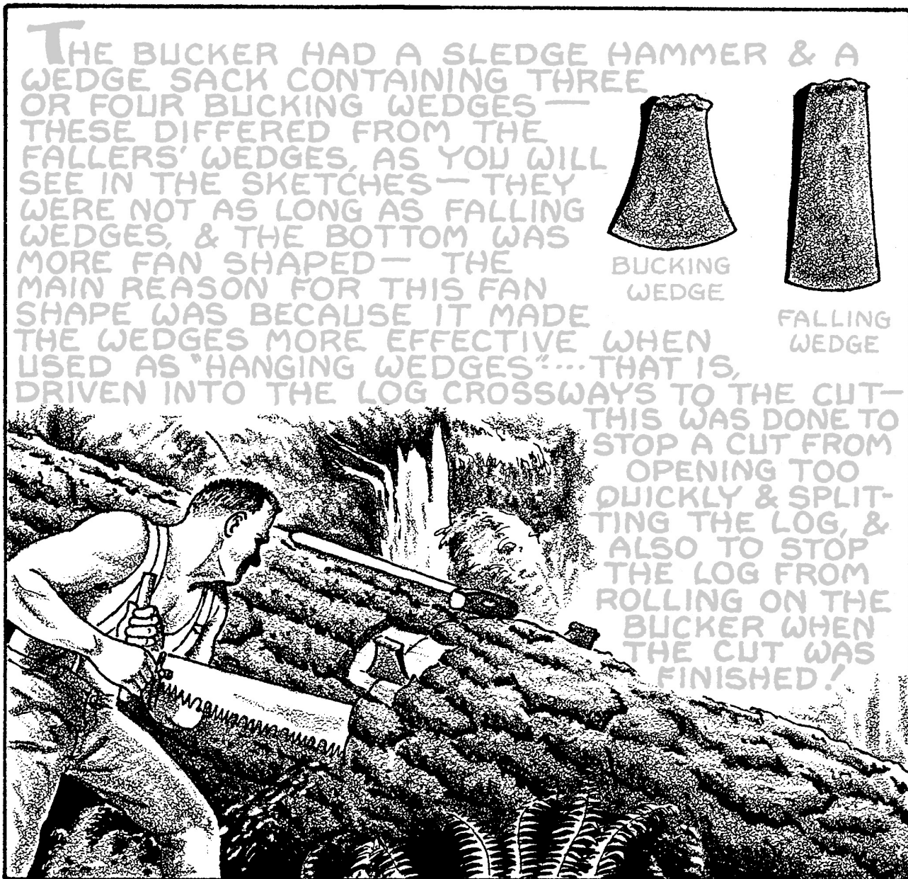
Figure 40—A bucking wedge being used as a hanging wedge. The wedge kept the cut from opening too quickly and splitting the log, and also stopped the log from rolling on the bucker when the cut was finished.—Now You're Logging, by Bus Griffiths, with permission of Harbour Publishing, Madeira Park, BC, Canada
