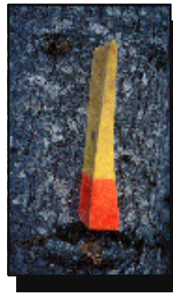
Figure 37—Triple-taper wedges allow a short wedge to provide as much lift as a longer wedge, but require more force to drive.
