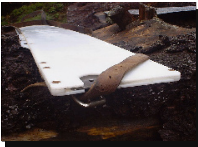
Figure 33—The sheath is made of \frac{3}{16} -inch high-density polyethylene, held together with countersunk copper rivets.—Photo used with permission of Jim Thode, Lewis County Chapter of the Backcountry Horsemen of Washington.
