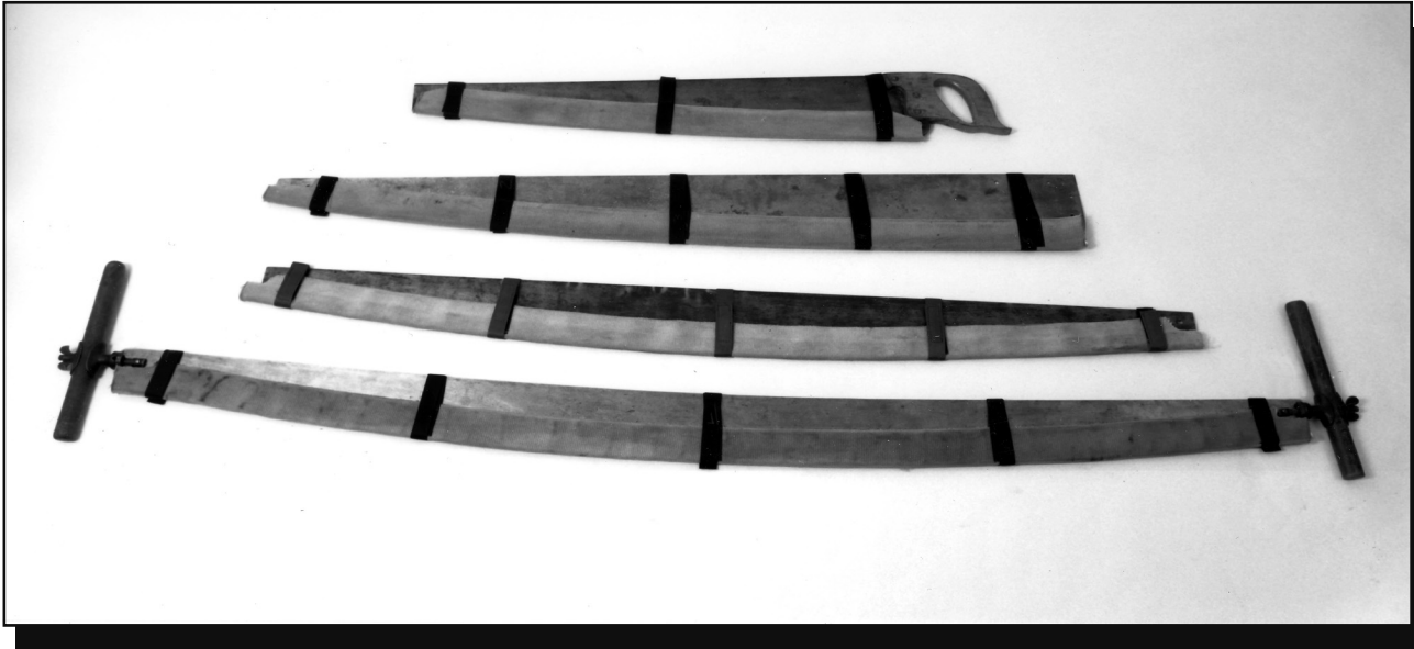
Figure 27—MTDC developed this saw sheath. The guard is made from 1½-inch discarded firehose using nylon straps and hook-and-loop fasteners.
