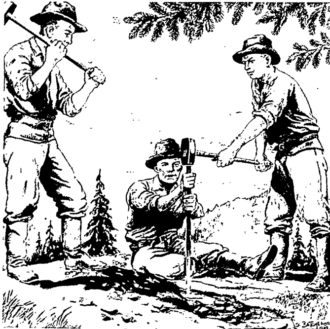
'Down hole' double jacking, early 1800's.
