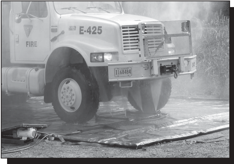
Figure 3—The underbody washer uses high pressure and a large volume of water to thoroughly wash mud, dirt, and debris from under the vehicle. The nozzles oscillate for complete coverage.
