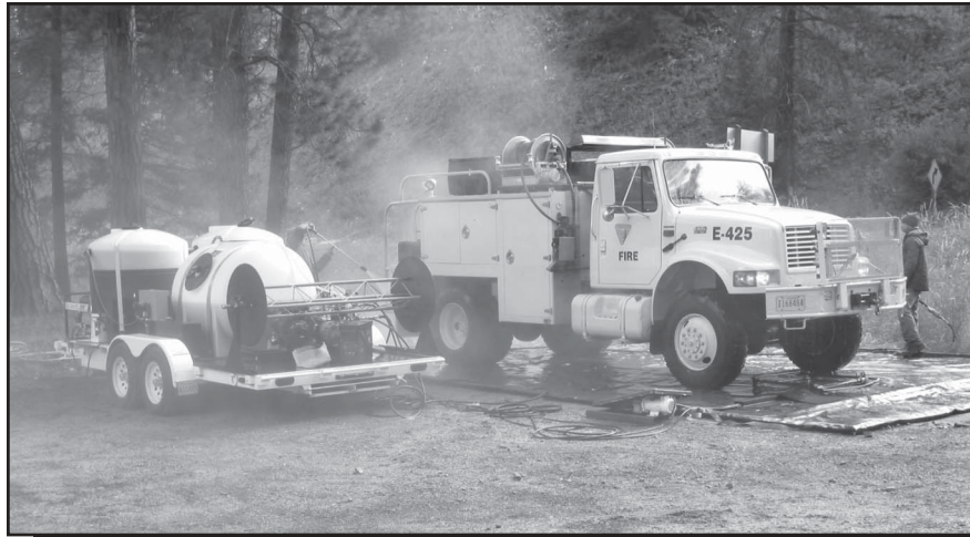
Figure 1—The MTDC prototype vehicle washer is used to wash a fire engine on the Bitterroot National Forest.
