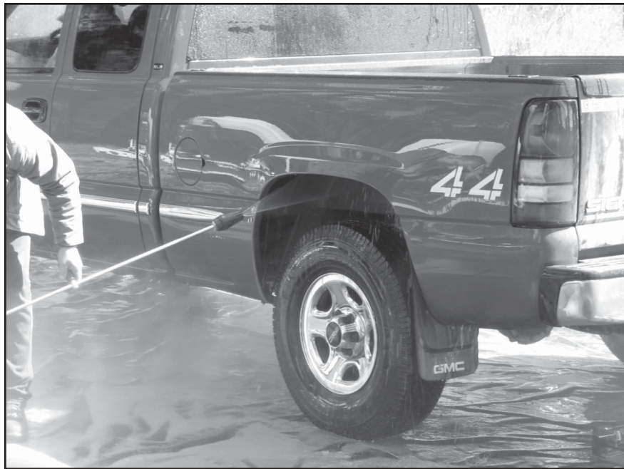
Figure 2—The hand-operated, high-pressure wands are used to thoroughly clean a vehicle's wheel wells, tires, sides, and bumpers where mud, dirt, spores, and weed seeds can collect.
