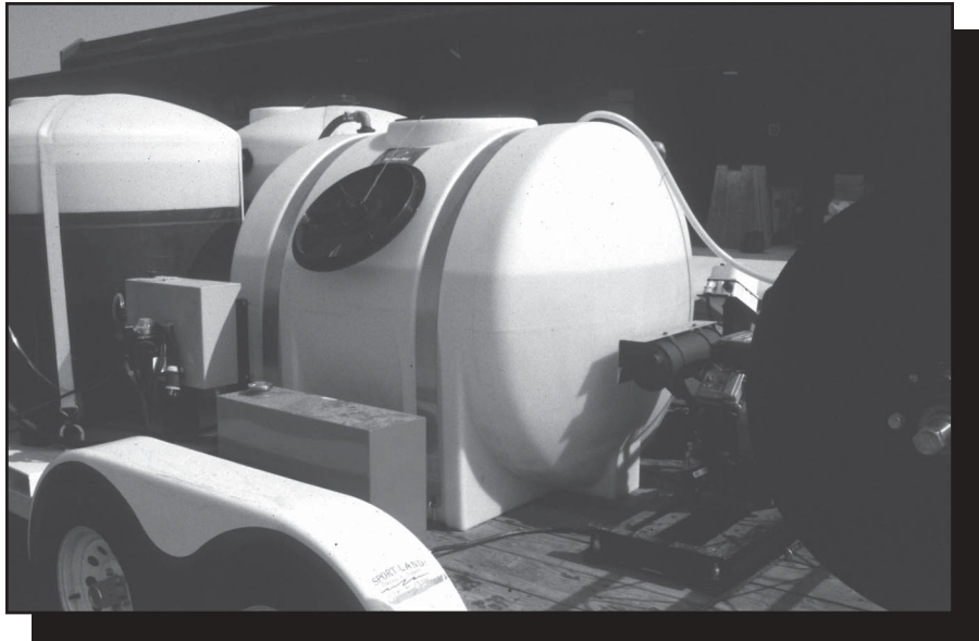
Figure 5—A 350-gallon tank is the main holding tank for the wash water.
