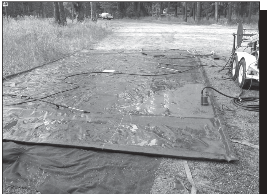
Figure 4—A 19- by 33-foot mat keeps the wash water where it can be recycled. Foam tubes are placed in slots along the mat's edges to create a barrier on all sides. The mat shown here was set up at the Bitterroot National Forest's Cathedral Fire in August 2002. The wash water drained to the lower right corner of the mat where a sump pump drew water for filtering and reuse.
