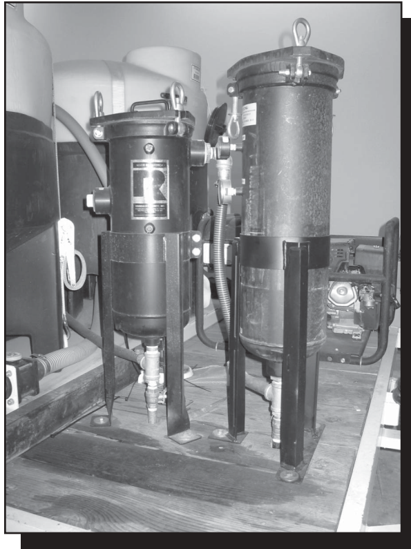
Figure 7—The filter housings are mounted on the trailer. Cloth or felt filters are used to remove particulate of different sizes, depending on the user's requirements. Typically, 20-micron filters will remove most noxious weed seeds while 3-micron filters can remove particles as small as fungal spores.
