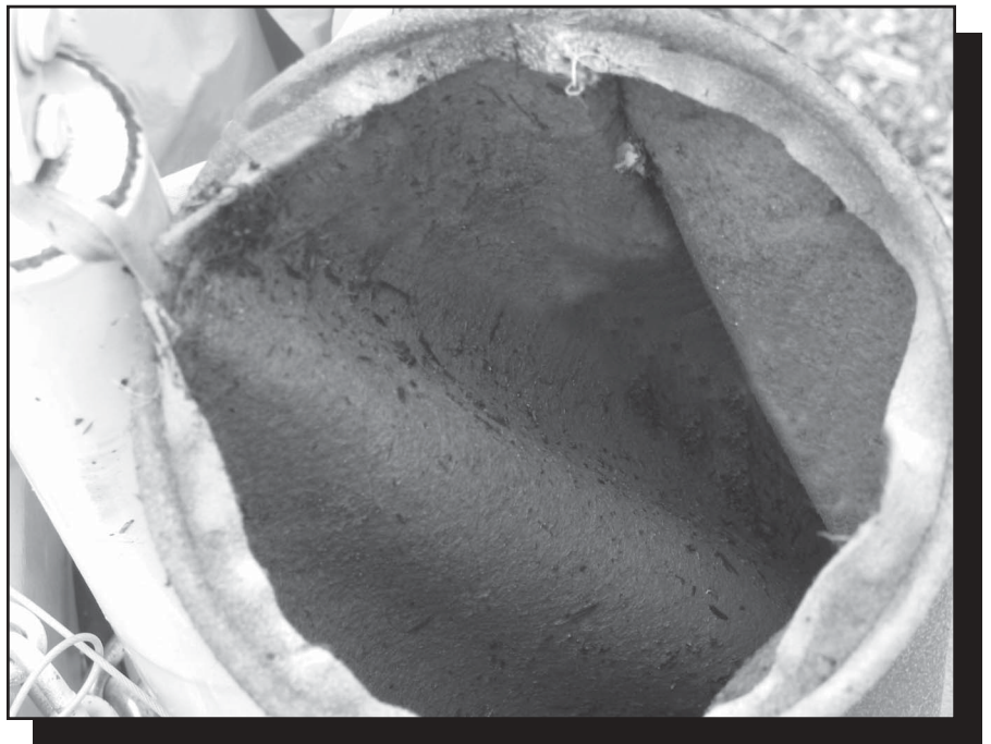
Figure 9—Filters collect noxious weed seeds and other debris from the wash water.
