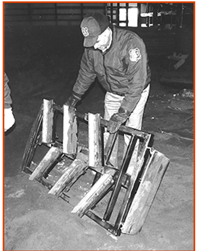
Figure 27—Dick Dufourd inspects “Big Bertha.” Its aggressive cutting action and weight are too much for an ATV to handle, but it works great in sandy soil when towed by a tractor.
