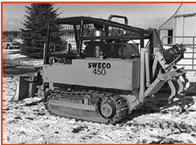
Figure 21—The SWECO 450 light crawler dozer has been upgraded to the 480 model.
