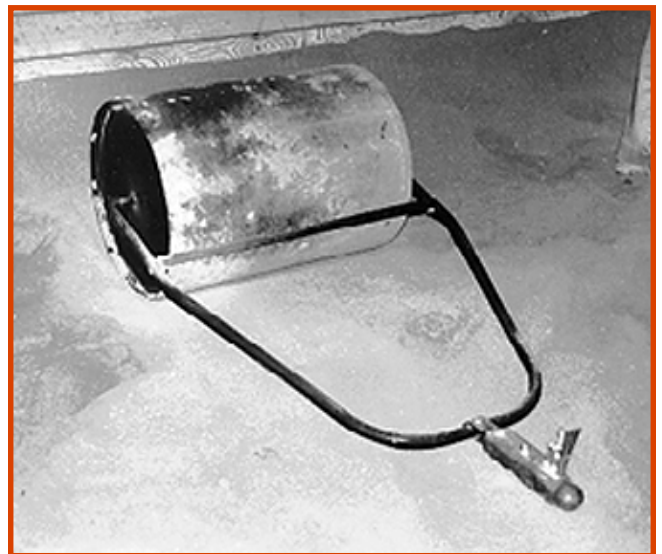
Figure 20—This garden variety lawn roller did not provide enough benefit to make it worthwhile for trail grooming. Pulling it is a waste of time.
