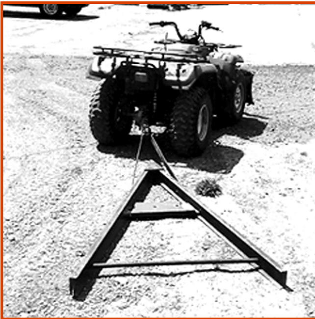
Figure 18—The V-shaped drag moves material to the side of the trail, a disadvantage.
