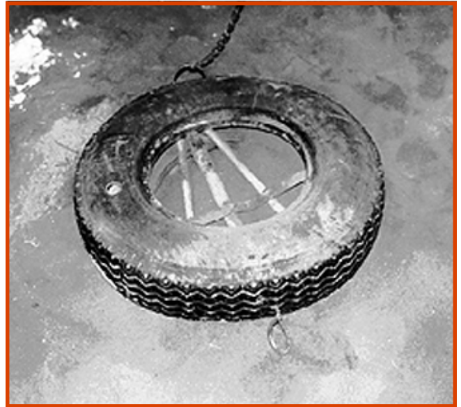
Figure 16—Tire drags with various configurations of one, two, or three tires help to provide a smooth, finished surface to the trail.
