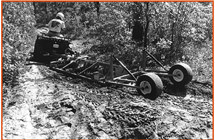
Figure 11—Due to its length and width, the Ultra Light Terrain Grader had a hard time negotiating corners.
