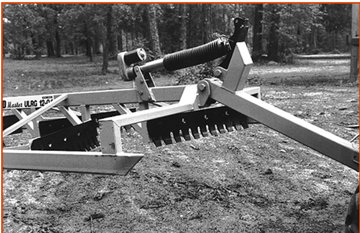
Figure 10—An electric actuator on the Ultra Light Terrain Grader lifts the front end to the desired level, setting the depth. Four angled serrated grader blades plus a rear straight grader blade pull soil to the center of the trail.
