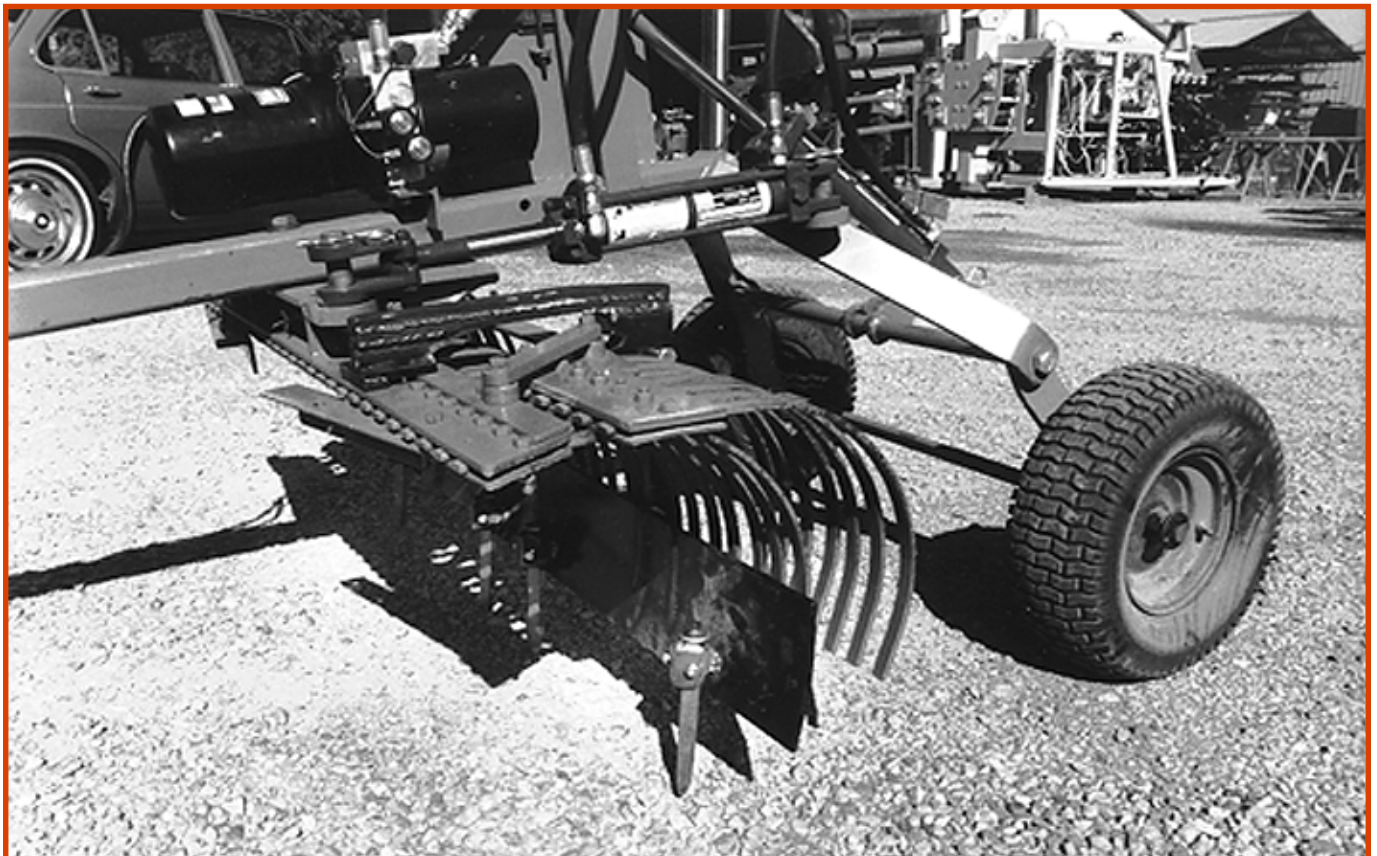
Figure 7—Ripper teeth attached to the scraping blade in an untested third prototype. The ends of the 6-foot (1.8-m) rake were hinged (center) to narrow the rake for trails and widen it for roads.
