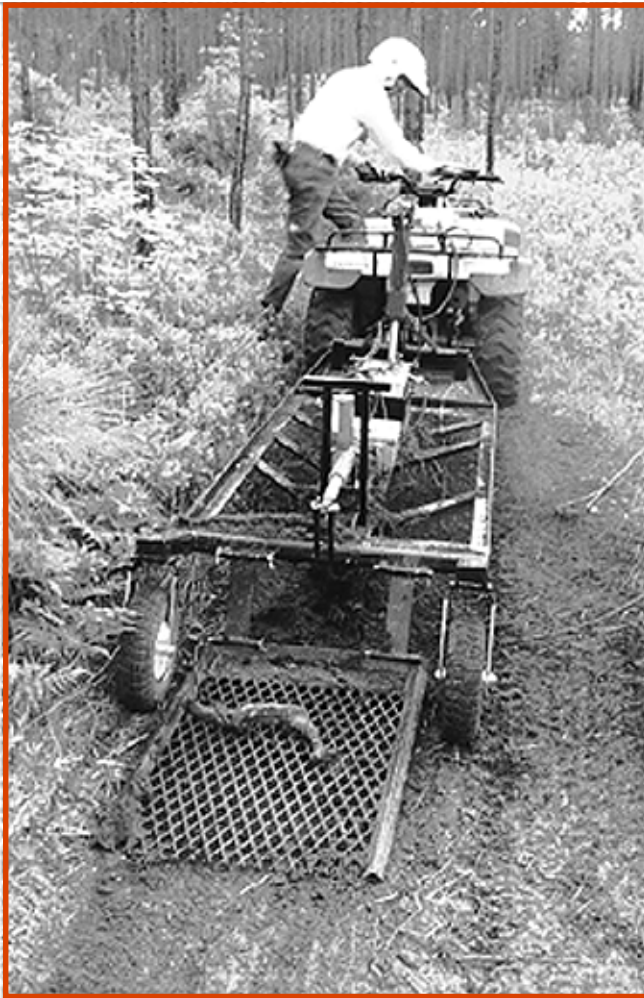
Figure 8—MTDC's version of the Deschutes Trail Drag. The original was only 28 inches (71 cm) wide, a better width for trails than this one, which is 34 inches (86 cm) wide. Angled blades on the drag provide a cutting action, pulling in loose tread material to the center of the trail. A straight blade on the rear, and a beavertail metal grate behind the rear wheels, smooth out the graded material.
