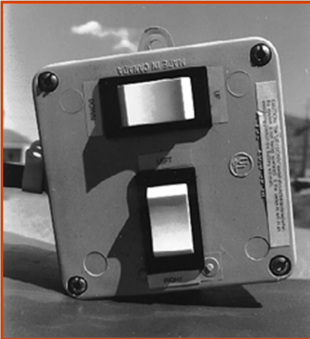
Figure 4—Control switch for the hydraulic power pack angles the rake and raises and lowers the wheels.
