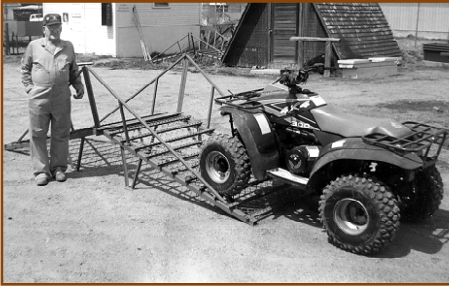
Figure 5—Carl Stoddard poses with the Caribou Trail Cattle Guard he fabricated in Montpelier, Idaho. Recycled steel fenceposts work fine as tread rails. MTDC modified the design shown here slightly to strengthen and widen the decking. The plans in Appendix B show the changes.
