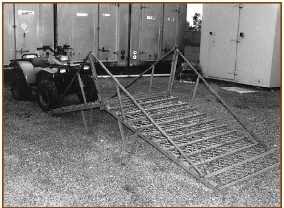
Figure 6—The two halves of the Caribou Trail Cattle Guard bolt together easily. Chain-link fencing keeps people from slipping through, but still discourages cattle.
