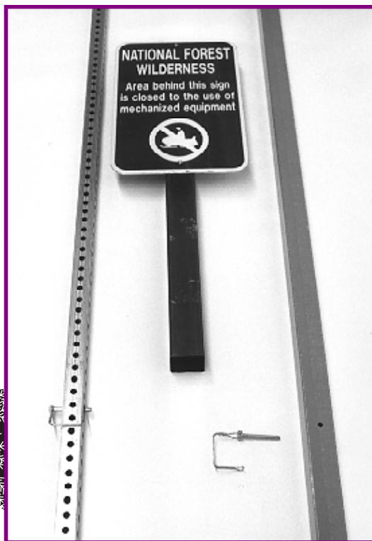
Figure 16—MTDC's steel and Extren plastic telescoping signpost system. The Extren plastic cost too much for us to recommend this system even though it is satisfactory otherwise. Telescoping two pieces of steel tubing is less costly.
