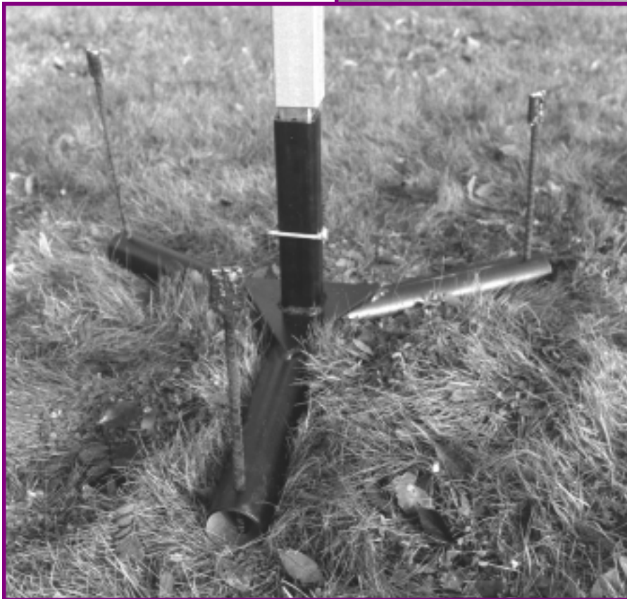
Figure 15—Gary Weigel designed this portable base. It is easily fabricated and can be customized to fit round or square posts. This base was used for MTDC's telescoping PVC signpost system (above), and also for the square tubular steel and Extren signpost (at left).
