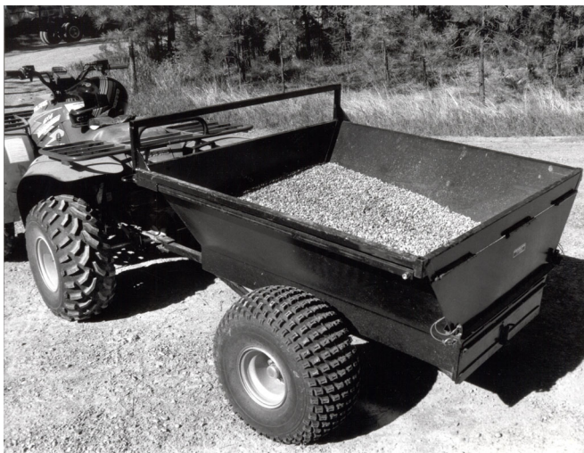
Figure 2—This maximum recommended load of 800 pounds of gravel fills the trailer less than half full.
