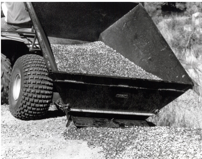
Figure 6—Gravel flow was uniform and adjustable.
