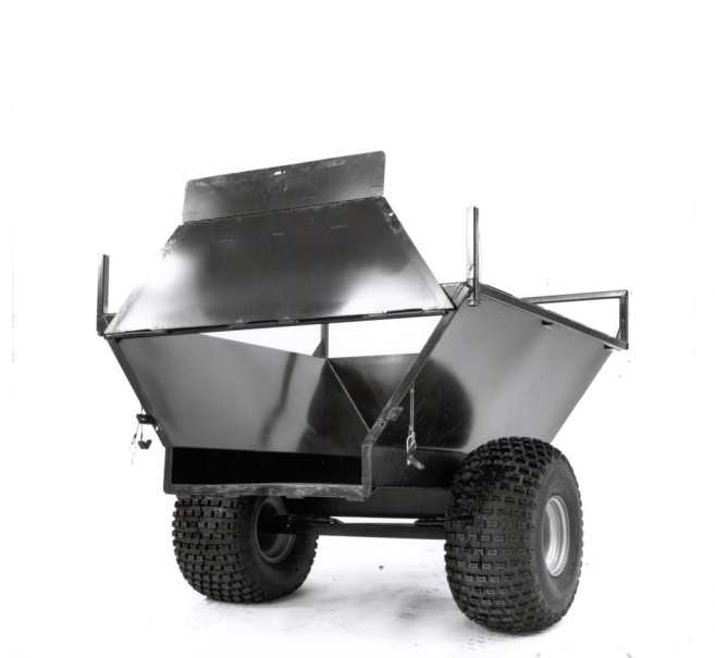
Figure 7—The entire tailgate can be lifted as shown or removed altogether.
