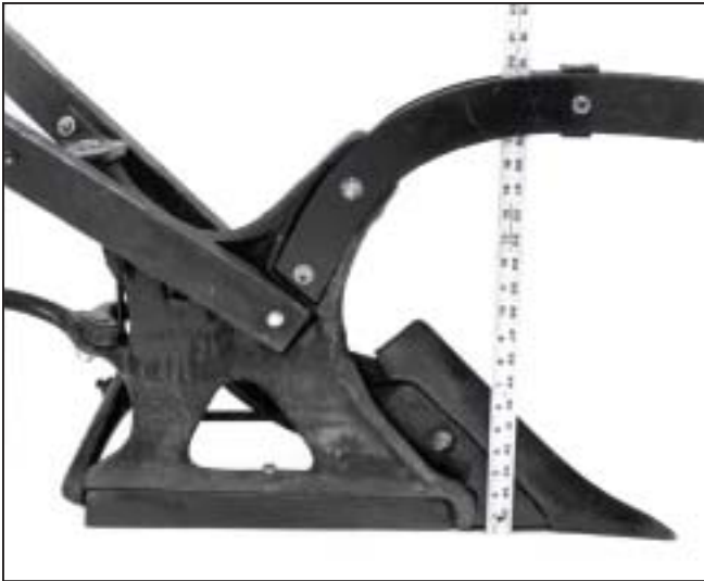
Figure 7—Vulcan plow showing about 1¼ inch of bottom suction.
