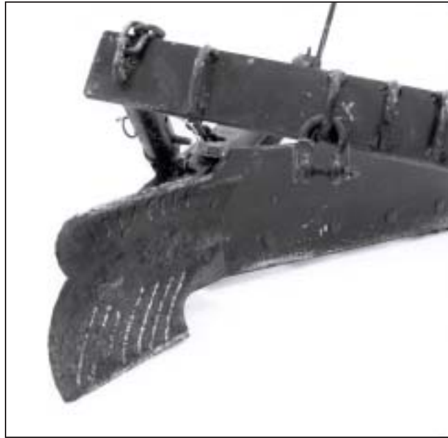
Figure 34—Blade on the MTDC combination plow and grader, fabricated from well casing.
