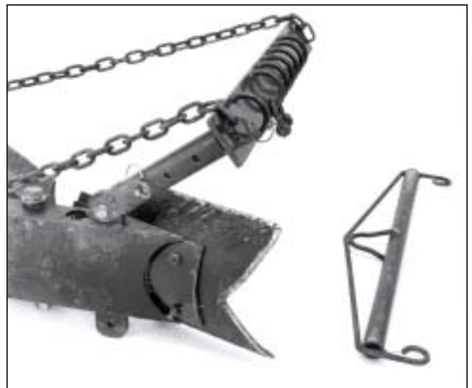
Figure 27—Closeup of the point and hitchbar with single tree of the MTDC combination plow and grader.
