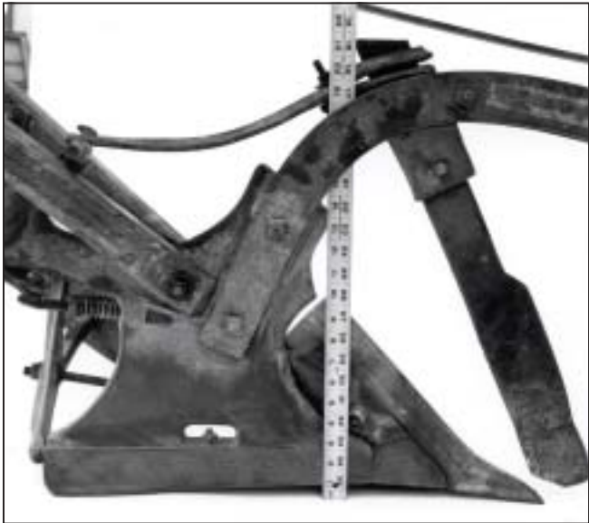
Figure 9—Chattanooga plow showing about 7/8 inch of bottom suction.
