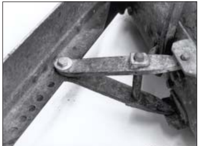
Figure 22—Beatty trail grader wing adjustment.
