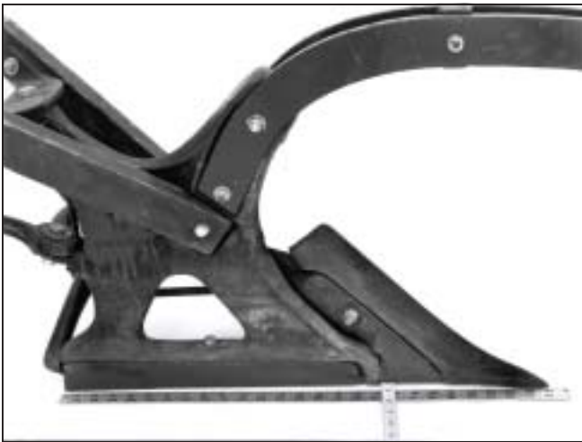
Figure 6—Vulcan plow showing about 1½ inch of hillside suction.
