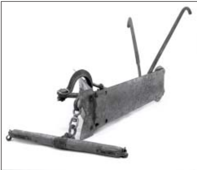
Figure 20—Beatty trail grader. Front view shows single tree, swivel clevis, hitchbar, and handles.
