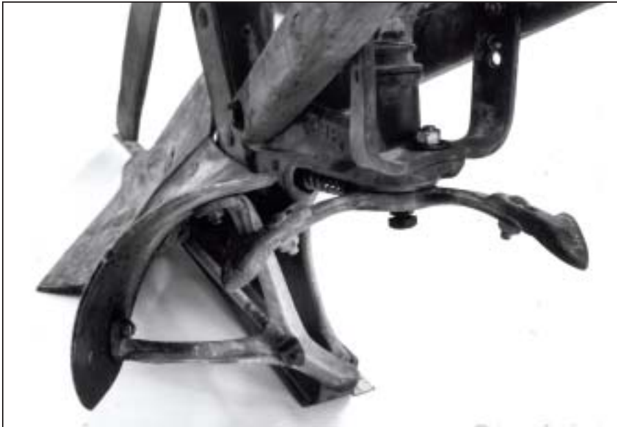
Figure 2—The latch on a hillside plow.
