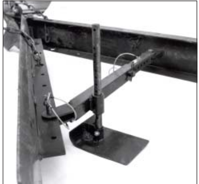
Figure 26—Shoe and wing adjustments of the MTDC combination plow and grader.
