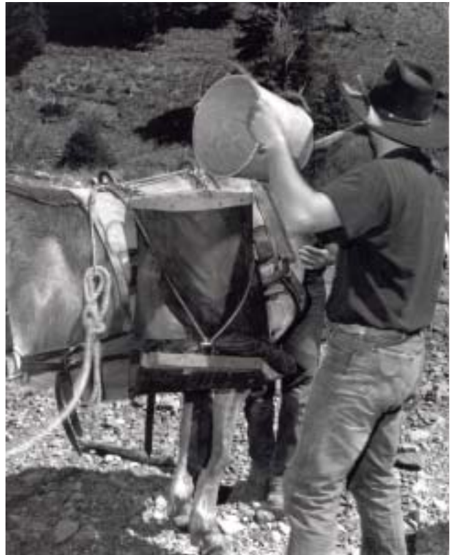
Figure 2.—This design is similar to the first, but has riveted seams and truck tarp fabric. Bags were filled one bucket at a time. Gloves should have been worn.
