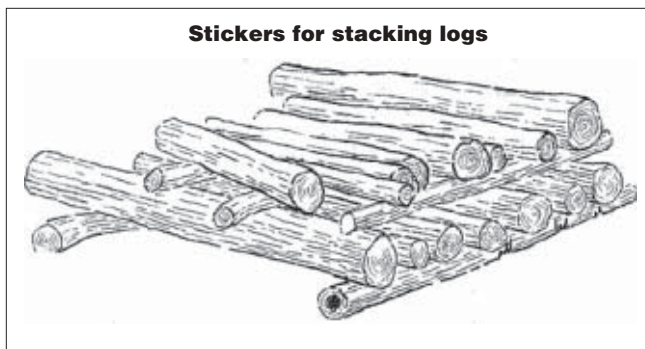
Figure 91—Stickers placed between layers of logs help the logs dry faster and reduce rotting.
