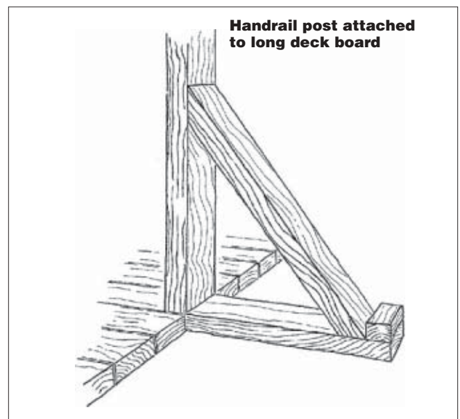
Figure 57—Attaching the handrail post directly to the decking requires long deck pieces to support an angle brace.
