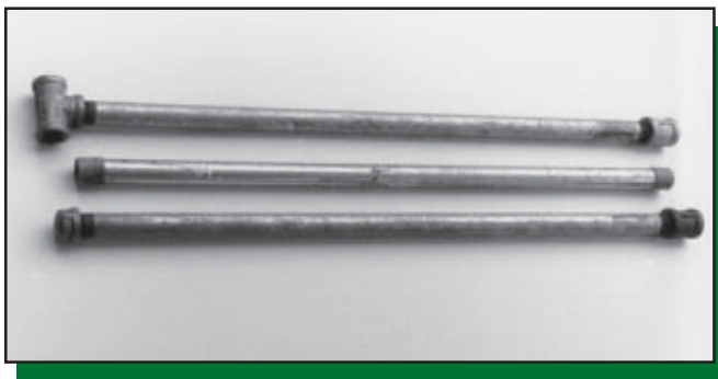
Figure 2—This sounding rod is inexpensive and easy to carry.
