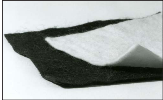
Figure 1—Geotextiles. Felt-like products are easier to work with than heat bonded, slit film, or woven products that have a slick surface texture. They are easier to cut and their flexibility makes them easier to place on curved trail sections.
