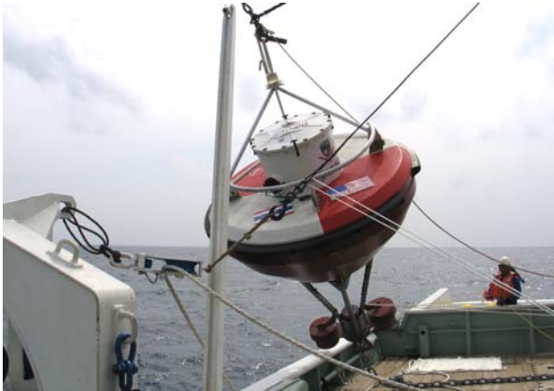
Technicians lower the DART tsunami detection buoy into international waters between Sri Lanka and Thailand.
