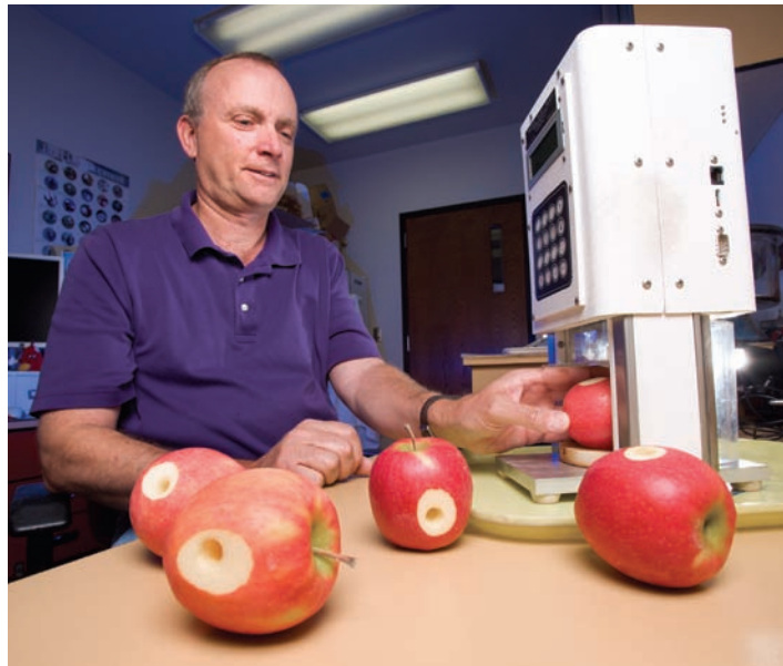
Technician David Buchanan uses a recording penetrometer to measure apple firmness, a key component of apple fruit quality.
