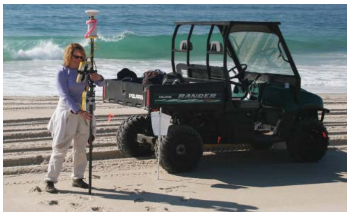
Hapke collecting real-time kinematic (RTK) global-positioning-system (GPS) beach profiles at Fire Island National Seashore as part of a topographic study of the beach and dune. Data have been collected seasonally in late March and late September for the past 3 years; data collection will continue for at least 2 more years. The NPS Northeast Regional Office in Boston is currently funding this research. Photograph by Mike Bradley , University of Rhode Island.
