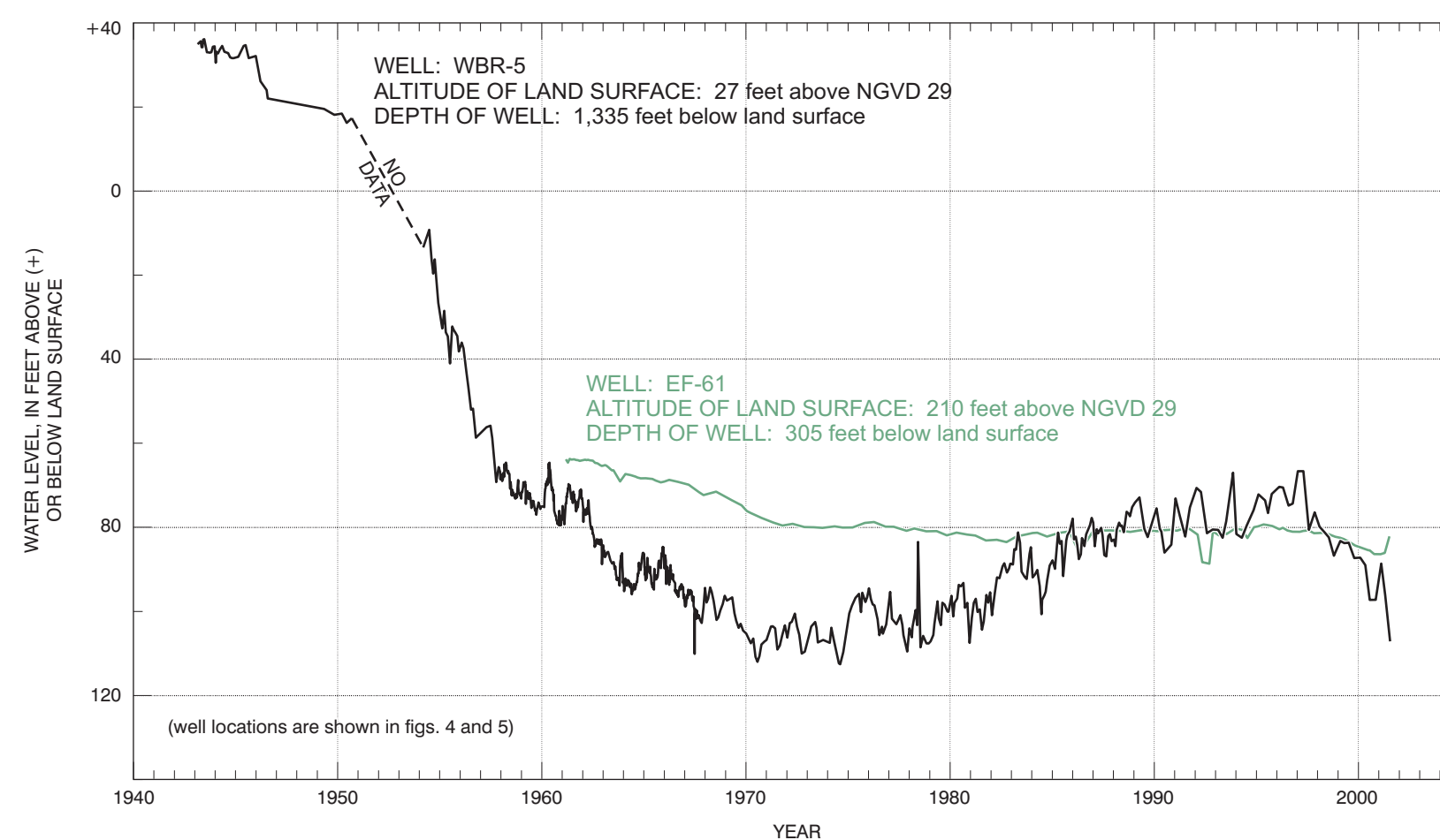
Figure 3. Water withdrawals from the "1,200-foot" sand and water levels in wells WBR-5 and EF-61 in the Baton Rouge area, southeastern Louisiana.
