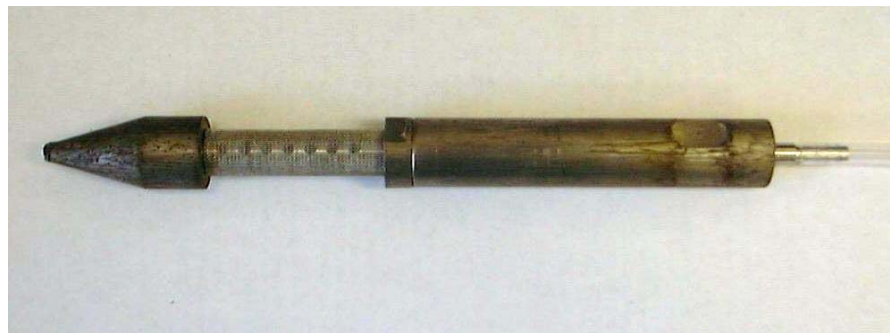
Figure 3. Probe used for AMS vapor sampling system
