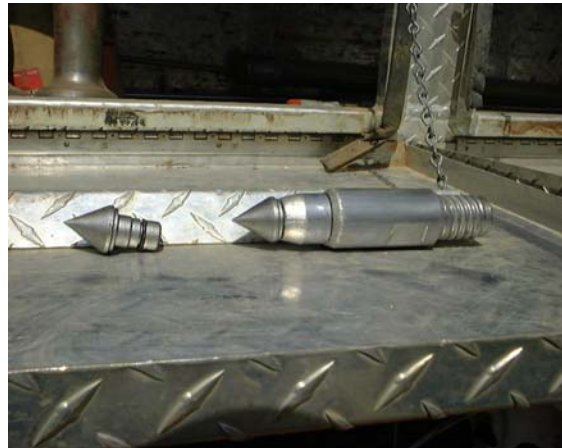
Figure 2. Probe used for Geoprobe PRT system
