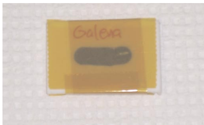
Figure C.7 Sample backfilled into opening of a Teflon block and secured with tape.
