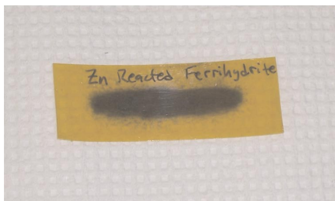
Figure C.6 Solid sample sandwiched between pieces of Kapton tape.
