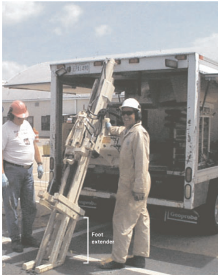
Figure 4.2 Geoprobe® in angle coring configuration (after Beck et al., 2002).
