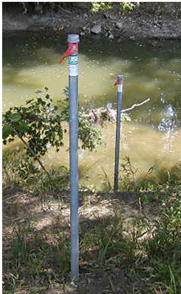
Figure 3. Photo of typical crest-stage gages. All sites have at least two pipes, one upstream and one downstream from the structure (bridge or culvert). Most sites have more pipes to cover the range of stages possible.
