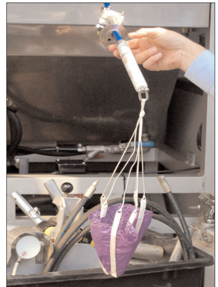
SSIS leak detection.
