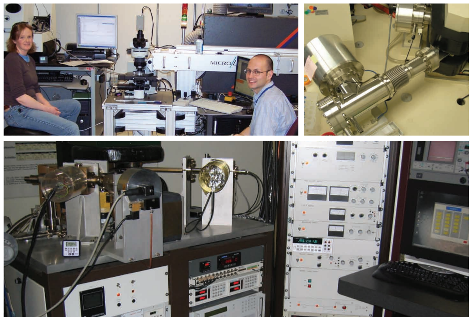
Figure 1. Analytical equipment housed in laboratories supported by the Evolution of Ore Deposits and Technology Transfer Project: laser ablation inductively coupled plasma mass spectrometer in the single fluid inclusion laboratory (top left), gas source magnetic sector mass spectrometer in the stable isotope laboratory (top right), magnetic sector mass spectrometer in the noble gas and active gas laboratory (bottom).
