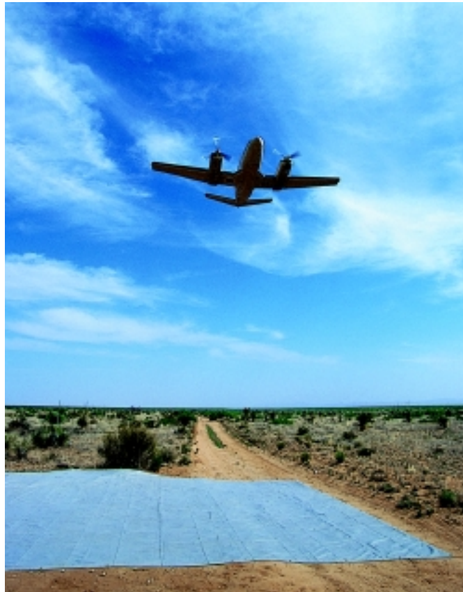
A reflective tarpaulin on the ground is used to calibrate the visible and infrared spectrometers aboard the Cessna.
