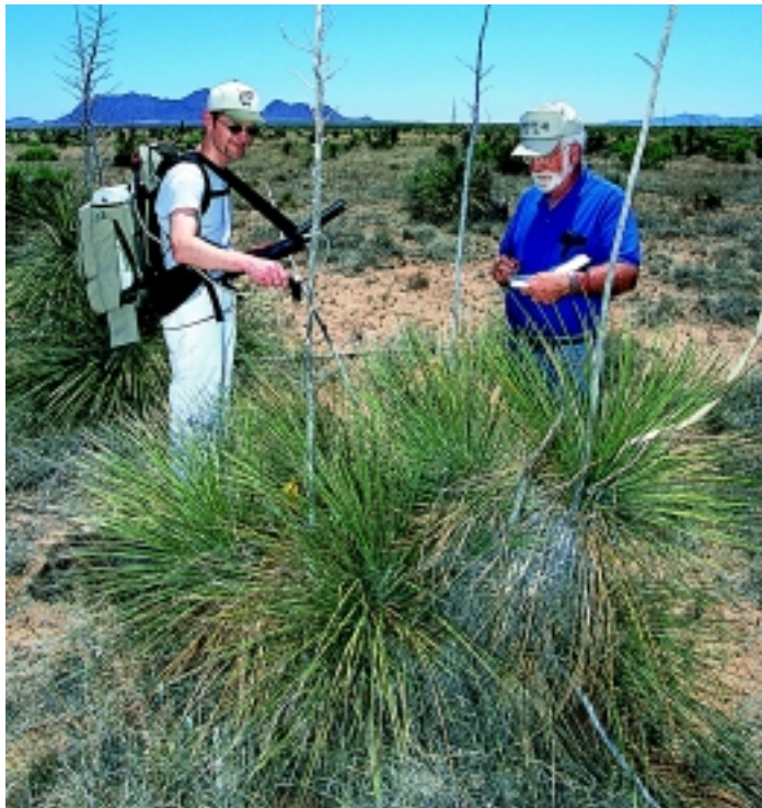
Jacobs (left) and soil scientist Jerry C. Ritchie take spectral reflectance measurements at the Jornada Experimental Range.
