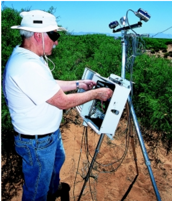
Schmugge sets up a thermal instrument to measure temperature on the Jornada Range.
