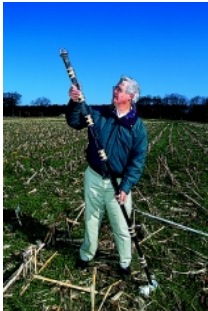
Probes like this one, held by soil scientist Tim Gish, monitor soil moisture. Soil-moisture data may one day help predict floods, drought, tornadoes, and hurricanes.
