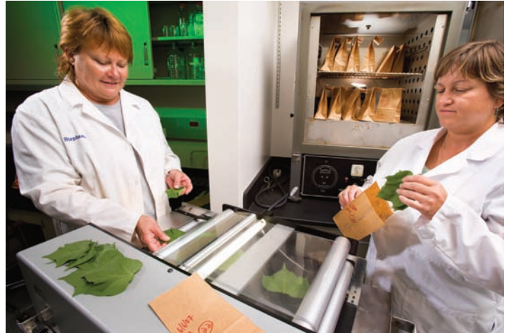
Plant technicians Stephanie Johnson (left) and Gwen Coyle record cotton leaf area measurements before processing the leaves for carbohydrate analysis.
