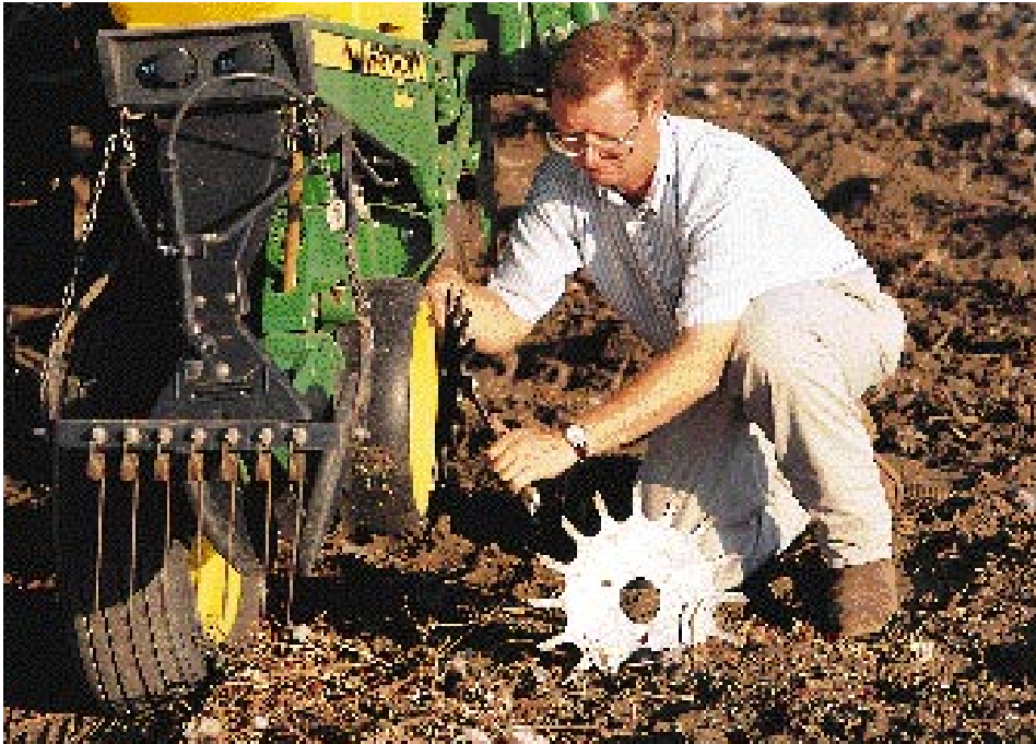
Agronomist Jim Smart is changing a planter's residue fingers—a tined wheel that moves dense crop residue aside so that seeds can be sown in the soil beneath. (K7520-3)
