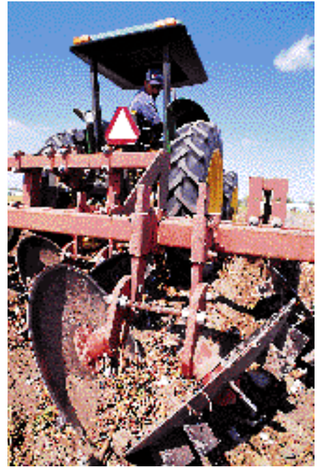
Field technician Emilio Chavez drives a tractor-drawn stalk puller that uproots plants after harvest. This prevents regrowth, water loss, and overwintering of pests in cotton and grain sorghum fields. (K7520-4)
