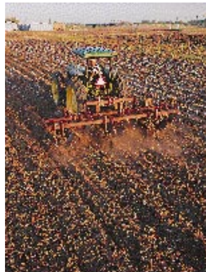
The stalk-puller attachment drawn through this cotton test field near Weslaco, Texas, by field technician Victor Valladares plucks out the whole plants, roots and all. (K7520-2)
