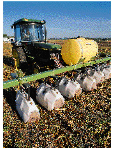
Hooded sprayers operated by field technician Victor Valladares direct herbicide just to areas between rows of grain sorghum. (K7520-7)
