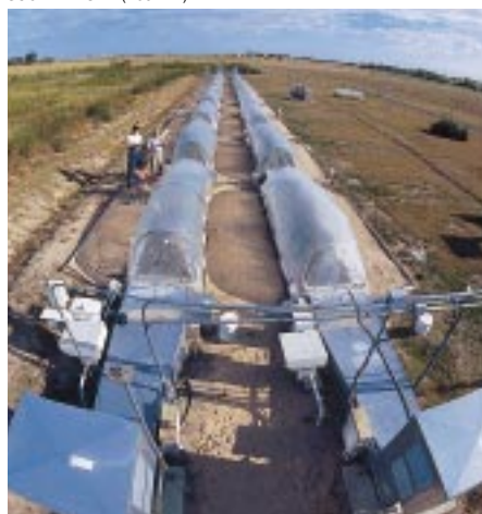
An aerial view of the two CO 2 -gradient tunnels. In the tunnel on the left, plants grow under present-day to ice age CO 2 concentrations, while those in the tunnel on the right grow under CO 2 levels of today up to those predicted for 2050.
