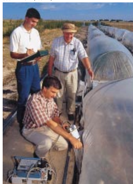
Rangeland scientist Justin Derner (left) and ecologists Wayne Polley (foreground) and Hyrum Johnson measure soil CO 2 emissions in the CO 2 -gradient tunnel system.
