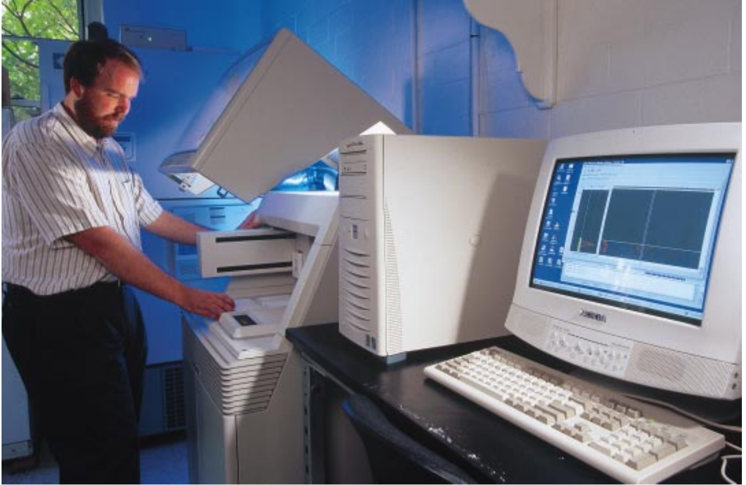
The high-capacity DNA sequencer being loaded by geneticist Curt Van Tassell will increase the number of genetic markers available for screening in the dairy population.
