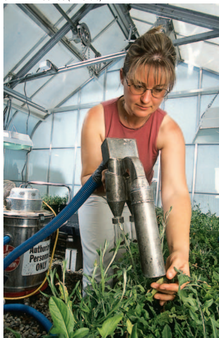
California Department of Food and Agriculture lab assistant Viola Popescu uses a cyclone spore collector developed at the Fort Detrick lab to harvest inoculum from plants at the CDFA greenhouse in Sacramento.
