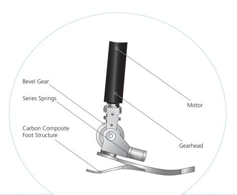
Our goal is to design an ankle-foot prosthesis that would mimic a normal walking gait and simulate natural joint function. We have conducted extensive studies of the human ankle to model its kinematics in order to provide the design specifications of this biomimetic ankle-foot prosthesis.
