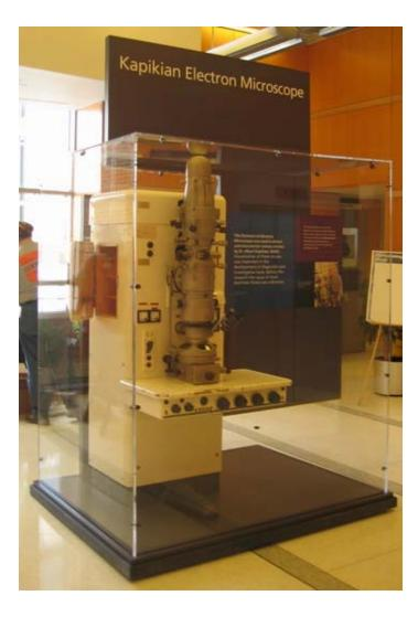
This Siemens 1-A Electron Microscope was used to detect and characterize the Norwalk virus, hepatitis A, and rotavirus by Dr. Albert Kapikian, NIAID. The microscope is now on display in the lobby of Building 50 (See p. 2).
