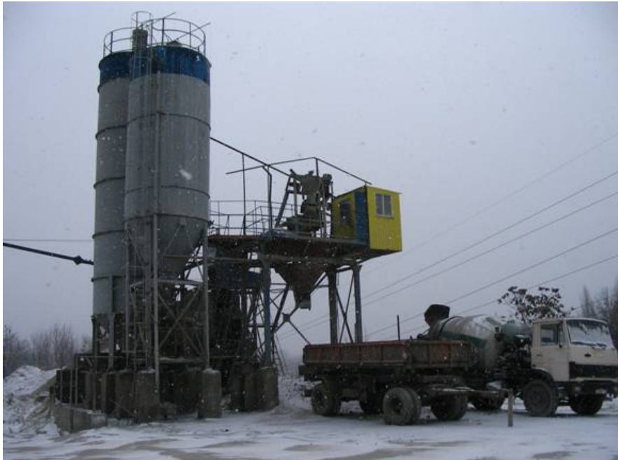
Photo of a cement maker that was modernized using the proceeds from a USAID guaranteed loan. This upgrade doubled the equipment's production capacity and improved the quality of the concrete produced, enabling the borrower, a construction company, to expand into larger and more lucrative construction projects. (Rostov-an-Don, Russia; January 19, 2006)
