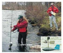
Amy Wehnke, USGS hydrologic technician, wades into a stream to measure streamflow using a current meter. Sandy Ward, USGS hydrologic technican standing on the shore, records the streamflow data Amy is measuring.
