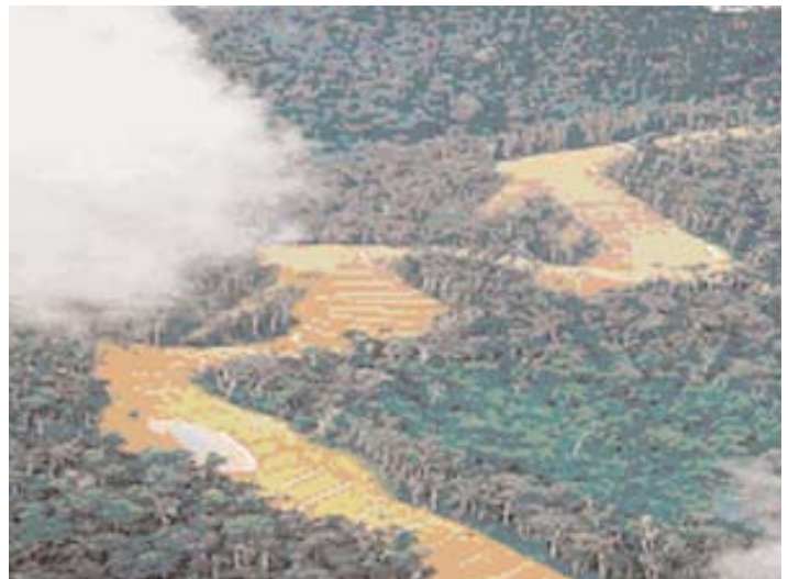
ROW with permanent erosion control.
