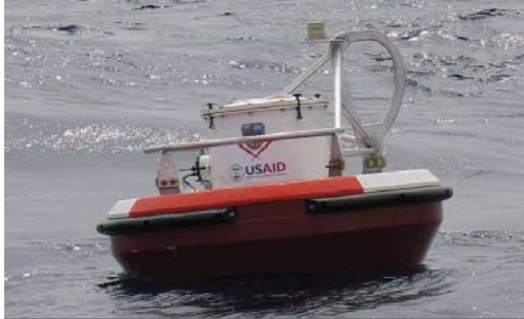
A Deep-ocean Assessment and Reporting of Tsunamis detection instrument, part of the Indian Ocean Tsunami Warning and Mitigation System.
