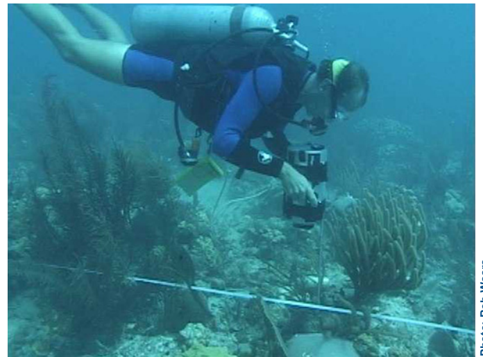
Diver using a sonar positioning system and video camera to record transect data in the U.S. Virgin Islands
